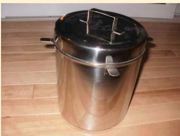
Water goes inside the container and the lid is secured. The charcoal burns for about 45 mins, after the charcoal goes out the unit can remain sealed for a further 15 minutes to complete cooking.
